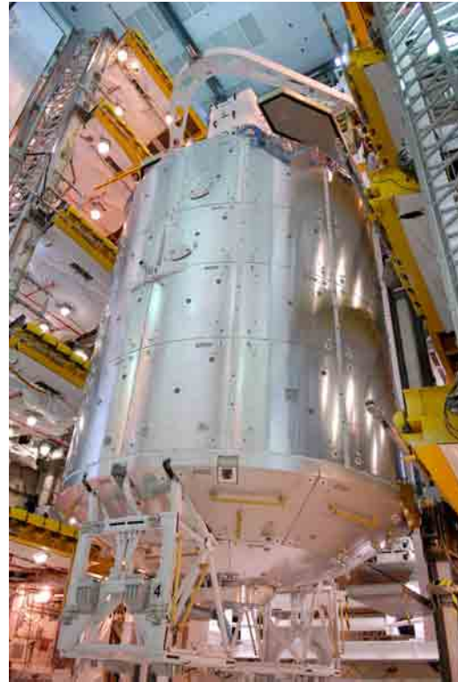
Fig. 6. Columbus laboratory ready for loading into a cargo bay of Atlantis US space shuttle. Two ARISS antennas are clearly visible in the upper part of the Columbus.
