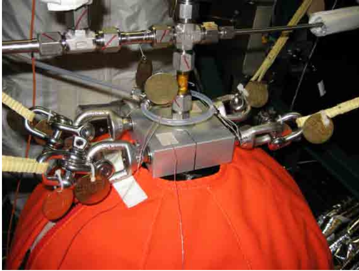
Figure 8. LN2 Spray Bar over Aluminum Support Block
