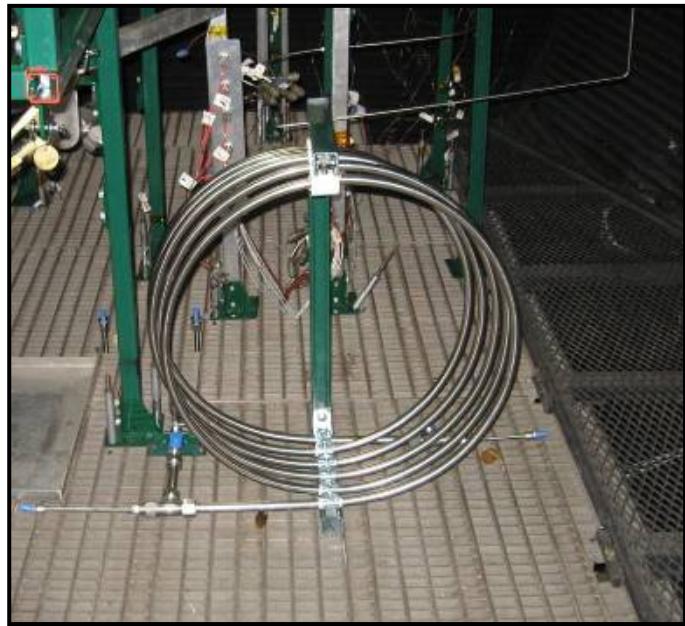
Figure 7. Tube-in-tube LN2 Heat Exchanger
